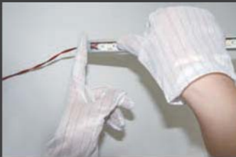
3.Put the end cap onto the profile and press gently to fix it.
