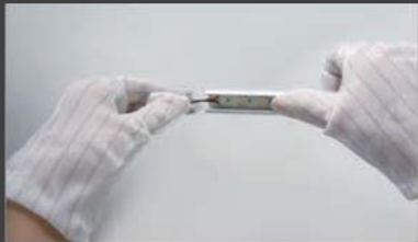
2.Take out the power cord through the hole on the end cap.
