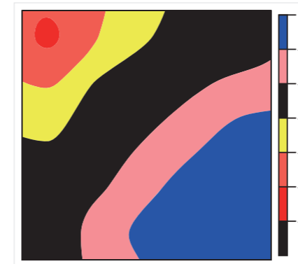
Horizontal illuminance (Grid) Average: 446 lx, Min: 409 lx, Max: 475 lx, Min/average: 0.917, Min/max: 0.861, Points: 5 x 5 (Relevant: all)
