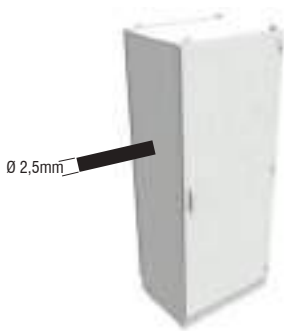
Protection against objects larger than 2,5 mm (device, cable)
