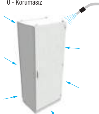
Second Figures: Protection against liquid objects 0-Unprotected
