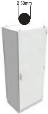
Protection against objects larger than 50 mm coincidental manual touch
