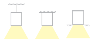
Suspended installation Ceiling installation Embedded installation
