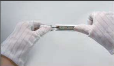
2.Take out the power cord through the hole on the end cap.
