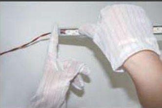
3.Put the end cap onto the profile and press gently to fix it.
